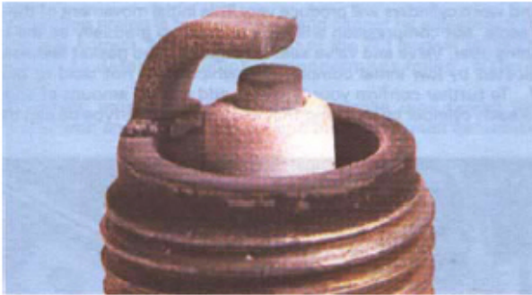
Spark plug conditions: A brown, tan or grey firing end is indicative of correct engine running conditions and the selection of the appropriate heat rating plug
