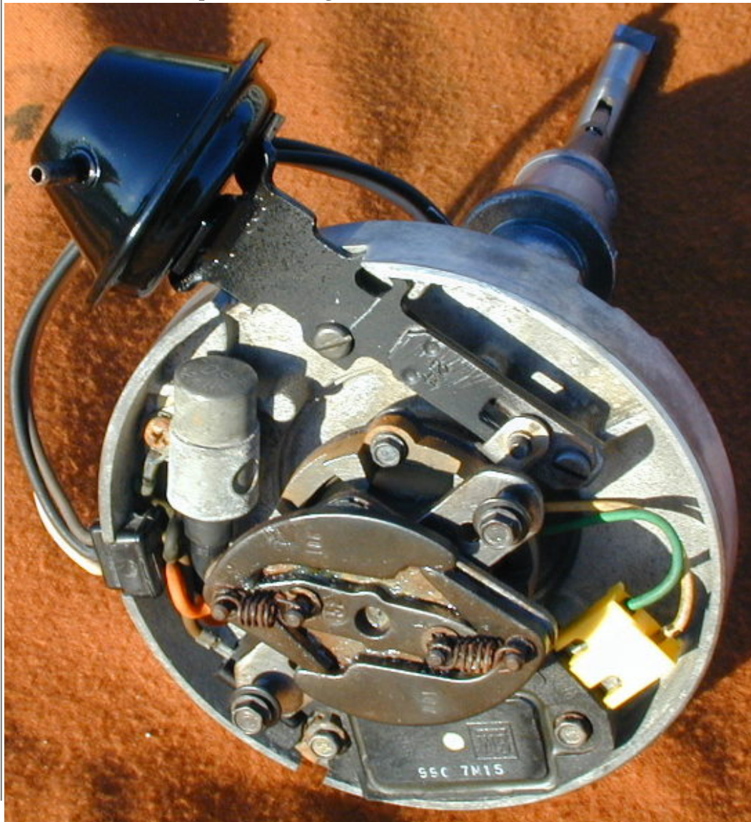
Early Electronic Ignition Distributor with dual points, centrifugal advance, and vacuum advance
