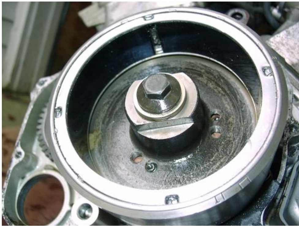
[Fig #2] : Two (2) Permanent North/South Pole Magnets On Flywheel Rotor
