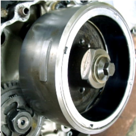
Pickup Magnet on Flywheel Outside
