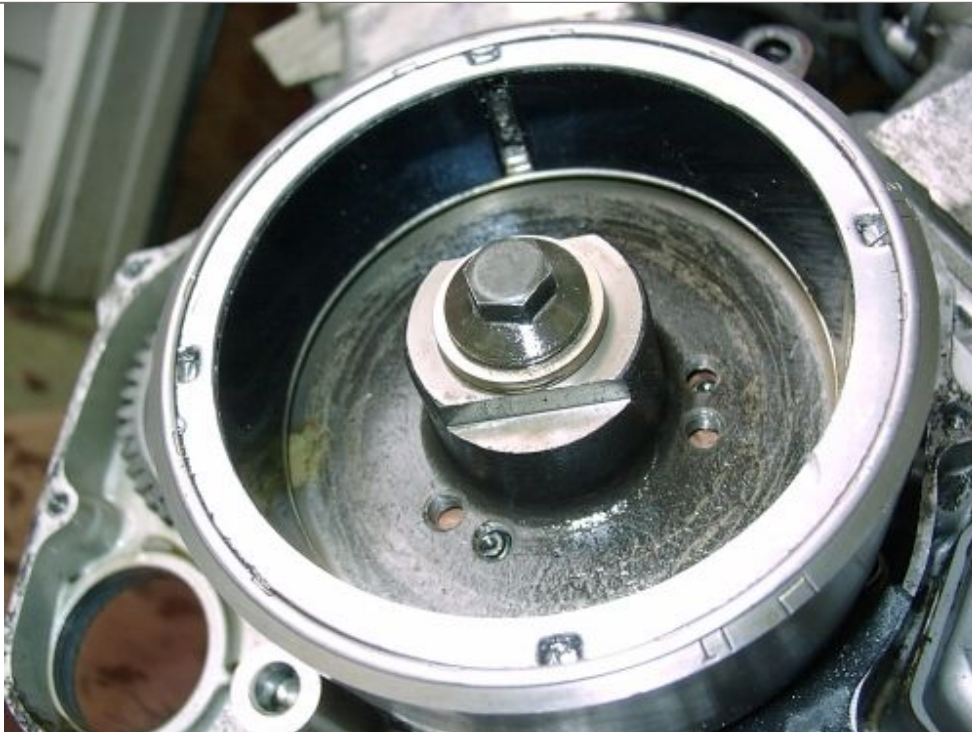
Flywheel with 2 magnets inside
